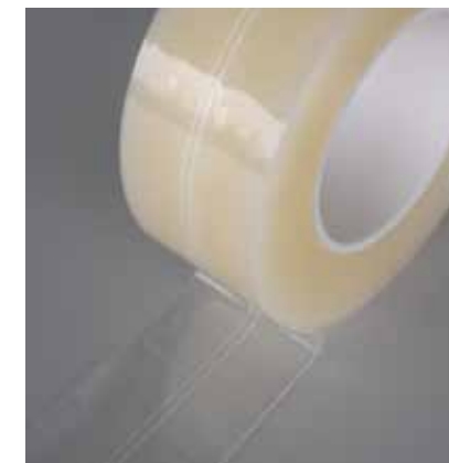
The bearing tape is double perforated. One side sticks to the formwork board, the other sticks to the ceiling bearing.
